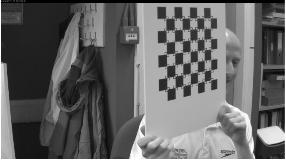
Figure 1. A typical image of a checkerboard showing the white space around the squares. This space is used to locate the board in the image. Each corner has been detected, and the square search area is superimposed on the image.
